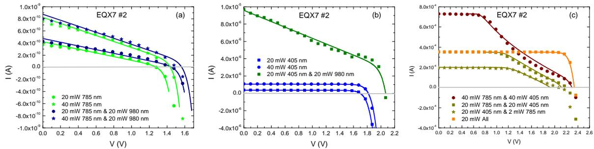
**Figure 1.** *I(V)* experimental results (symbols) obtained on a triple junction device. Laser powers used for the experiment are shown in the figure. The lines are the fits obtained with the numerical calculation.
