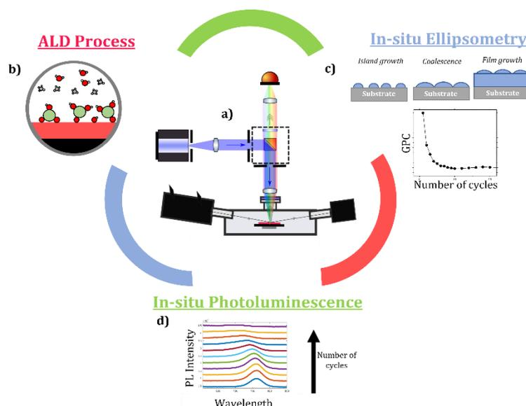
a) Experimental set-up with in-situ PL and ellipsometry in an ALD reactor b) ALD growth c) In situ ellipsometry - Thickness, optical constants and growth mechanisms d) In situ PL – Functionalization properties (passivation, carrier behaviour)
