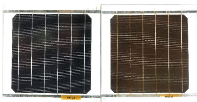
Fig 1: Comparison of monocrystalline modules with either low (left) or high (right) cut-off encapsulant after 4200 hours long UV aging
